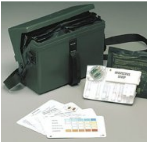
The M256A1 chemical agent detector kit used by the U.S. Army detects and preliminary identifies chemical agents on the field. (Source: U.S. Army)
